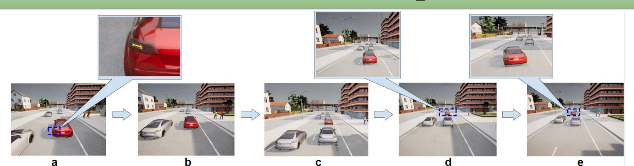
The ego vehicle took a sequence of actions in the interaction process to successfully merge left. (a) The ego vehicle intended to merge left. It turned on the left signal. (b) The surrounding vehicle on the left was not cooperative at first. The ego vehicle kept left blinking. (c) The surrounding vehicle on the left became cooperative, and the ego vehicle started to move left. (d) The ego vehicle kept moving left and found room in the left lane. (e) The ego vehicle successfully merged left.
